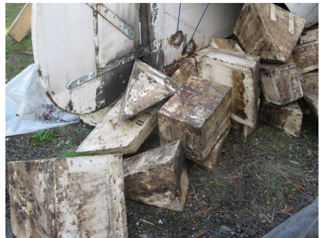
Some of the 'air case' flotation components found inside the hull
